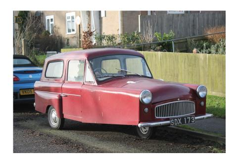
BOND MINI CAR 250cc Villiers 2 stroke. Max speed 50mph with following wind. 50% more wheels than my previous transport and I was out of the wind, rain and cold.
